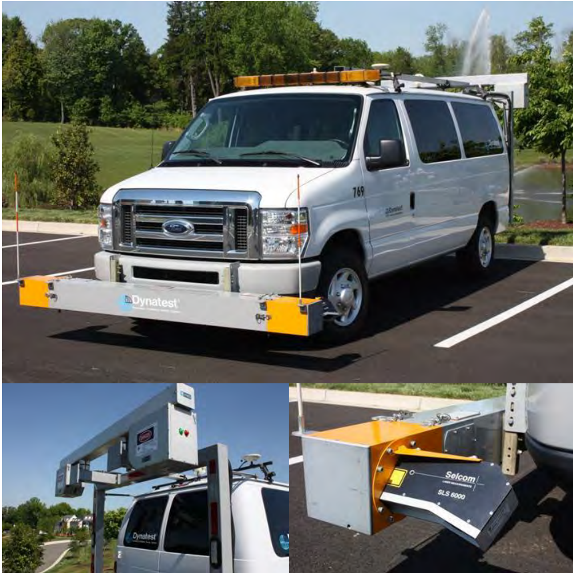
Figure 5 Dynatest PCSS Equipped with LRIS
